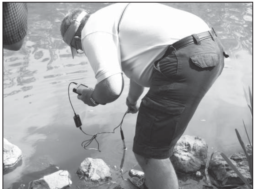
Agriculture teachers use graphing calculators and pH sensors to collect water quality data.
